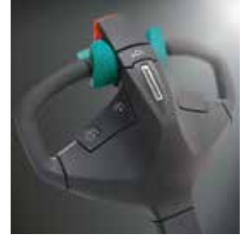
Easy and safe to manoeuvre: The safety control handle of the pedestrian trucks.
